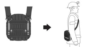
Shoulder belt should be placed in such a way that the buckle for adjustment and the free end of the belt be on the outside
