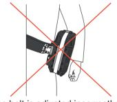
The belt is adjusted incorrectly
